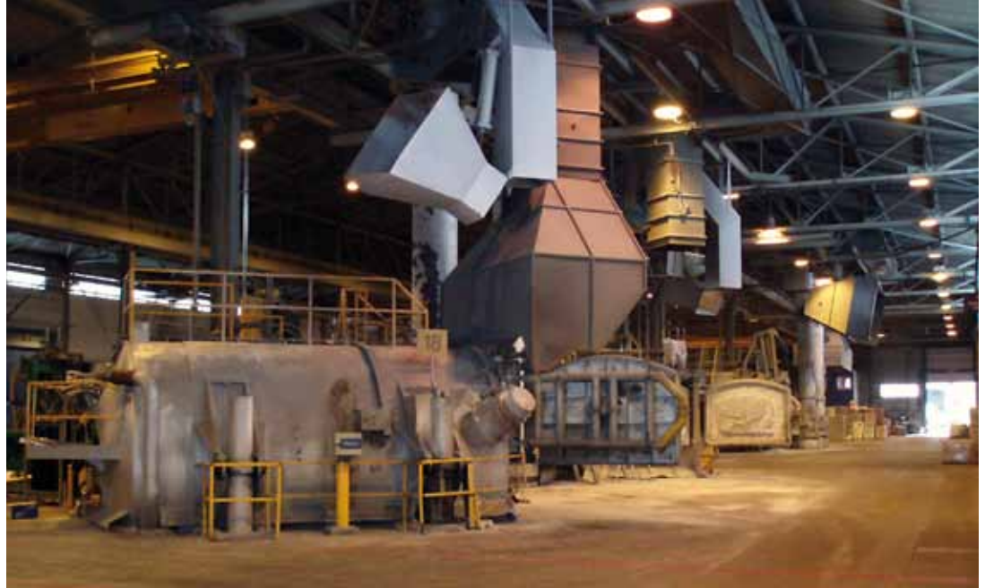
The two lines for primary foundry alloys production at Hydro Aluminum's Årdal works were converted to Low-temperature Oxyfuel in 2007 and 2008.
