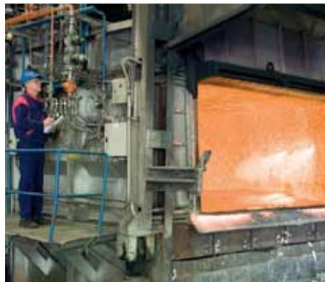
Going from conventional to Low-temperature oxyfuel, melt rates are further increased and dross reduced at SAPA Heat Transfer, Sweden.
